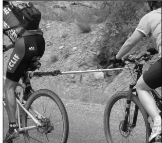
swing out approximately 75 degrees to either side. x2Cycle specifies this device should not be used when riding down
